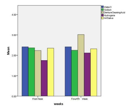
Figure (3) mean roughness (Ra) in Mm for COE-SOFT for the all solutions versus storage intervals
