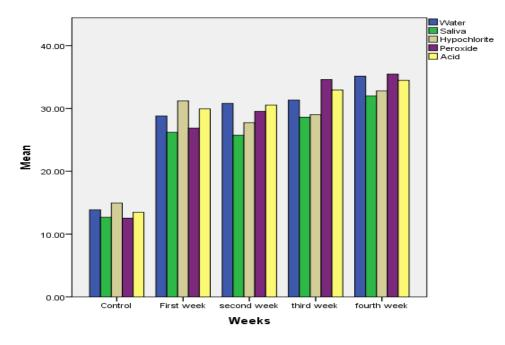
Figure (2) COE-COMFORT mean shore A hardness versus time intervals for the four immersion and control groups
