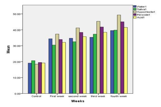
Figure (1)COE-SOFT, mean shore A hardness versus time intervals and the four immersion with control groups
